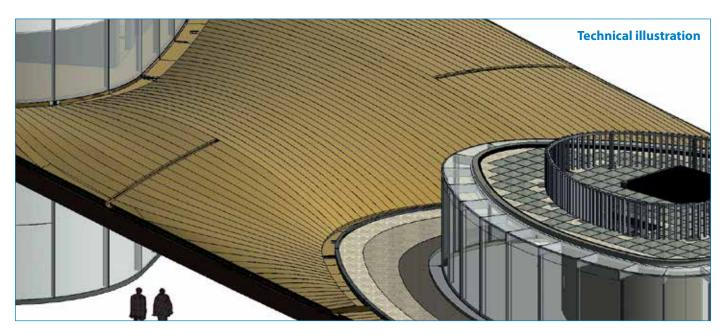
Kevin Turton, Design Manager at Kalzip®, said: "Our investment in computer-controlled manufacturing means we can transform computer-generated designs swiftly into reality. For the Greenwich Gateway Pavilions, we took 3D roofing sheet data extracted from the BIM model to schedule production of each unique Kalzip® XT component.
